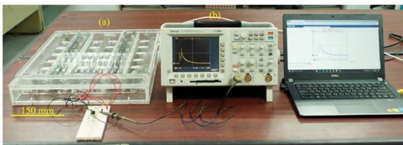
Fig. 11. A test setup showing (a) the energy harvesting floor tile and (b) the oscilloscope measuring the voltage (Tektronix TDS3032B).
