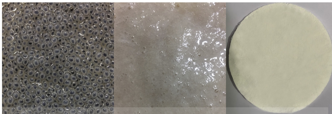
Fig. 2. Basil seed in different forms (a) swollen basil seed, (b) mucilage extracted from outer pericarp of the seeds and (c) BSM hydrogel sponge.
