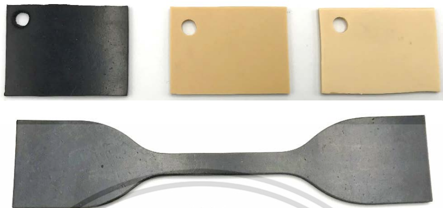
Figure 3.2 NBR1-commercial NBR, NBR2 and NBR3 from left to right (Upper), cut by die cut type C for tensile test according to ASTM D412
