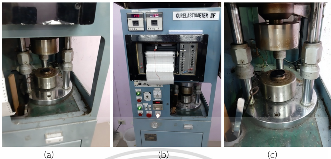
Figure 3.13 Pictures taken during cure test (a) specimen is placed in moving die rheometer for cure time test (b) moving die rheometer on progress and (c) specimen after cure time test.
