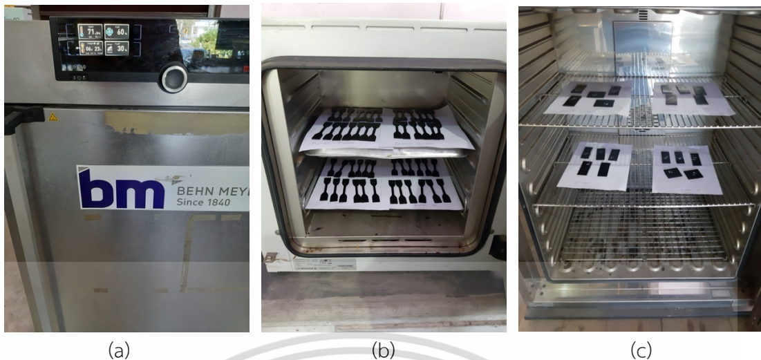
Figure 3.17 (a) Air oven used for accelerated aging, (b) specimens for tensile test in accelerated aging process, (c) specimens for hardness test in accelerated aging process.
