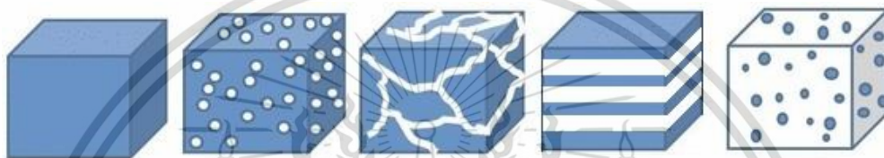
Figure 2.10 Phase morphology in an immiscible blend [24]
