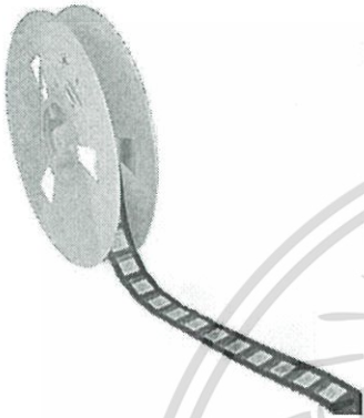
Figure 5: Reeled u-blox 6 modules
