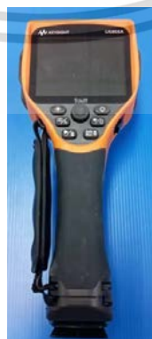
Figure 3.12 The thermal imaging camera equipment.
