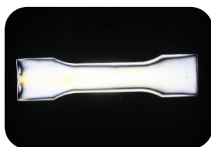
Annealing temperature tests of 90 °C and annealing time at 15 mins
