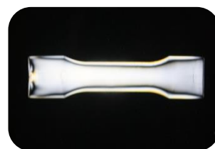
Annealing temperature tests of 90 °C and annealing time at 30 mins
