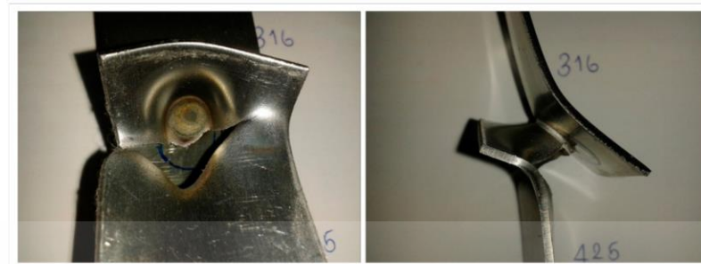
Figure 7. Tensile surface fracture of the pullout failure mode.
