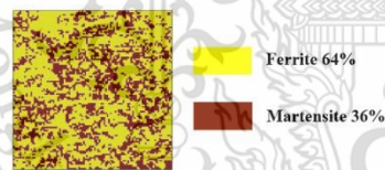
Figure 3. 2D RVE of the investigated steel.
