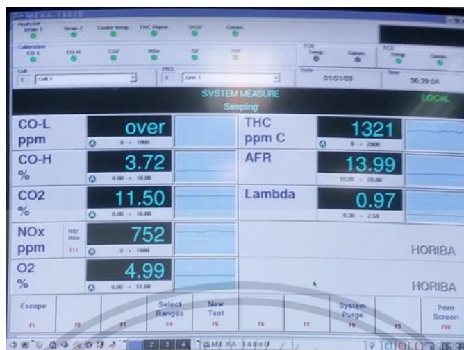
Figure 78 Horiba Mexa-1600D interface
