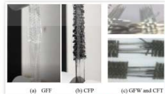
FIGURE 2 Appearance of the Fracture of fiber after tensile test (a) GFF while tensile test, (b) CFP while tensile test and (c) GFW & CFT after tensile test.
