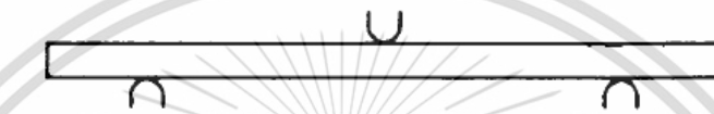
(c) Bending nose radius with 3.2 mm Figure 3.8 The testing method of flexural strength.
