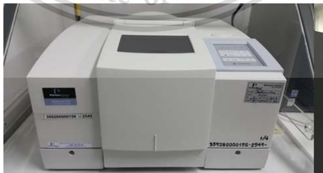
Figure 3.4 Fourier Transform Infrared Spectrometer (Perkin Elmer, Spectrum One)
