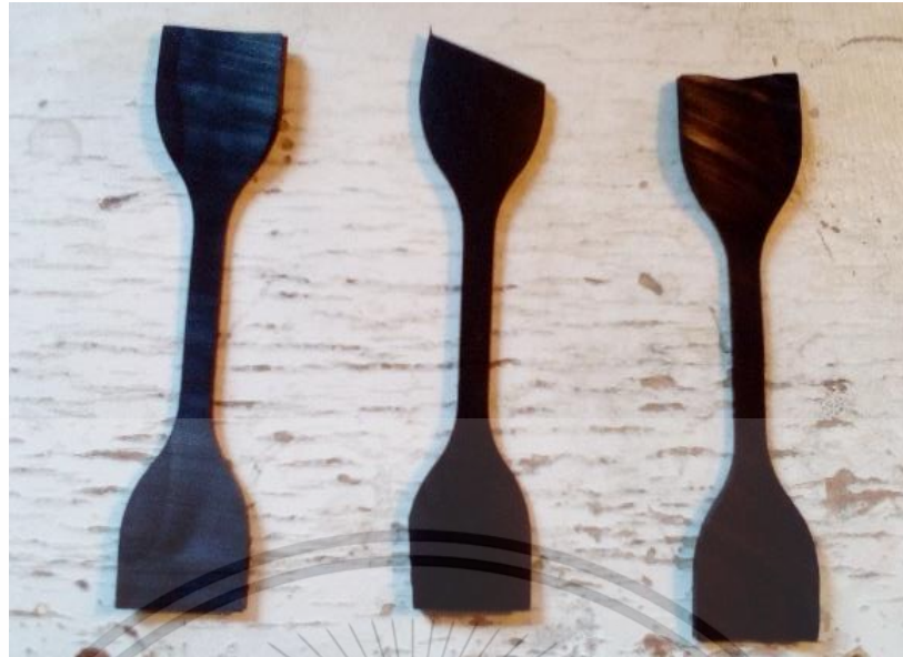
Figure 4.10 Dumbbell specimens from rubber materials.
