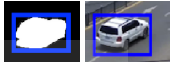
Fig. 6. Result of BLOB detection (a) Detected vehicle in binary image (b) Detected vehicle in real video's image
