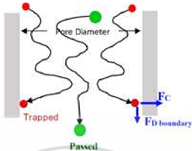
Figure 2.22 Trapping characteristics of PM in DPF filters [18]
