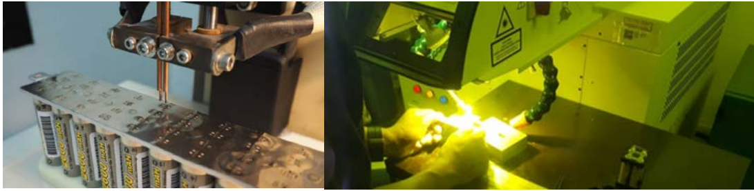
Figure 3.45 Spot welding and Laser welding technique
