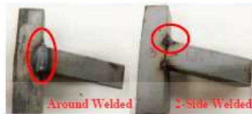
Fig. 22 Deformation comparison between Around welded and 2-Side Welded
