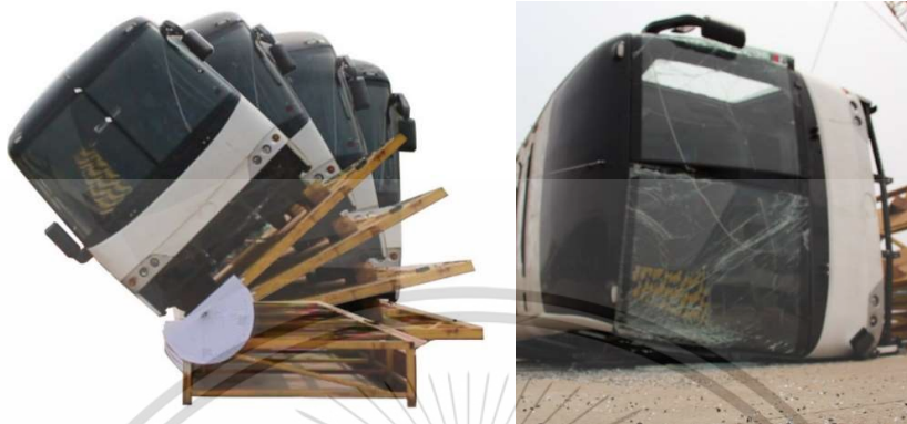
Figure 1.3 Full scale Rollover test
