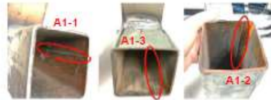
Fig. 15 Different seam welded positions on an internal surface of vertical structural steel member in T-joint specimens
