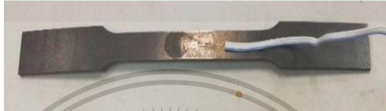
Figure 3.13 Strain gages with specimens for tensile test
