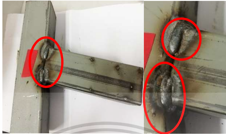
Figure 4.23 Deformation behavior for corner weld group 1 (Large size)
