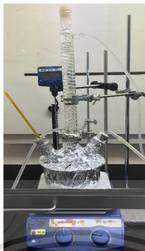
Figure 61. Schematic set-up of artificial ageing method with addition of ethanol.
