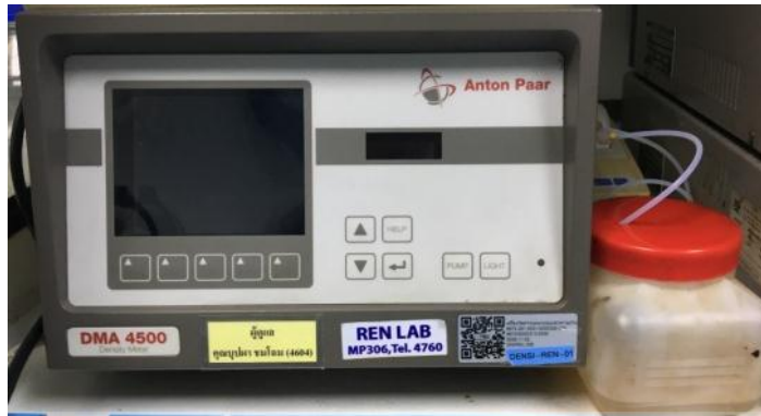
Figure 51. Digital density-meter (Anton Paar DMA 4500).
