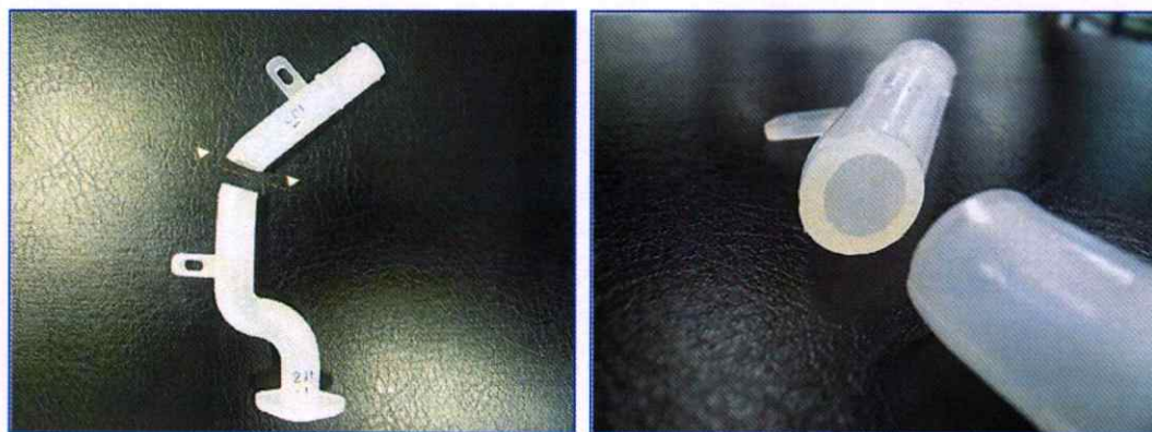
Figure 3.8 The location of sectioned part for determining the residual wall thickness
