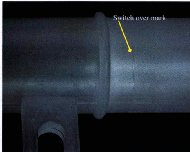
Figure 3.15 Visible surface defect of switch over mark as molded by Short-shot process of WAIM
