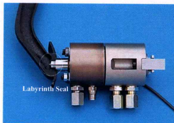
Figure 2.40 Water nozzle injecting direct into the mold cavity
