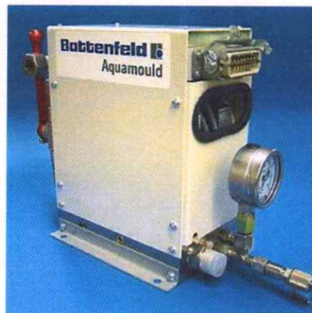
Figure 2.34 Water pressure and water control module
