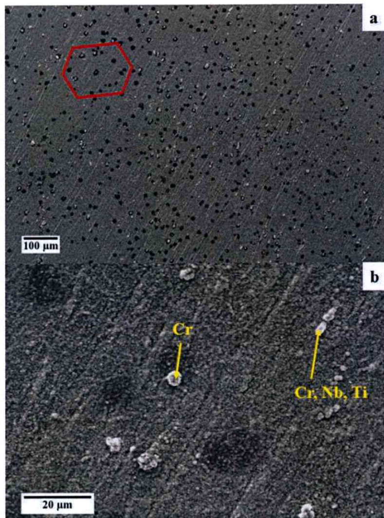
Figure 7.17 SEM images in SE mode of P.Ar-850+ox.4 when the magnifications were a). 100x and b). 1000x.
