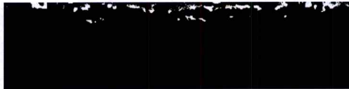
Figure 5.18 Binarisation of Si and voids (white phase) observed from the IG-nodule.
