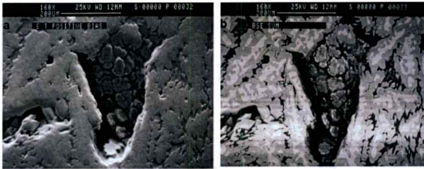
Figure 3.8 The comparison between a) a SE image and b) a BSE image for the same area of Ni alloy [19].
