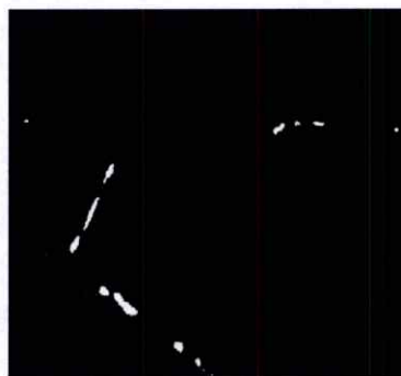
Figure 5.19 Binarisation of Nb phases (white phase) observed from the IG-nodule.
