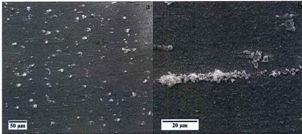
Figure 4.3 SEM images in SE mode of Bare 441 after high temperature oxidation (2 cm/s, 5% \text{H}_2\text{O} in \text{O}_2 , 800°C, 96 h) when the magnifications of the images are a) 200x and b) 1000x.
