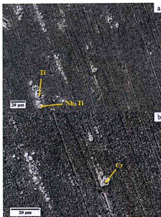
Figure 8.8 SEM images in SE mode of P.CO/CO 2 -250+ox.4. a). and b). show the different locations and their magnifications were 500x and 1000x respectively.
