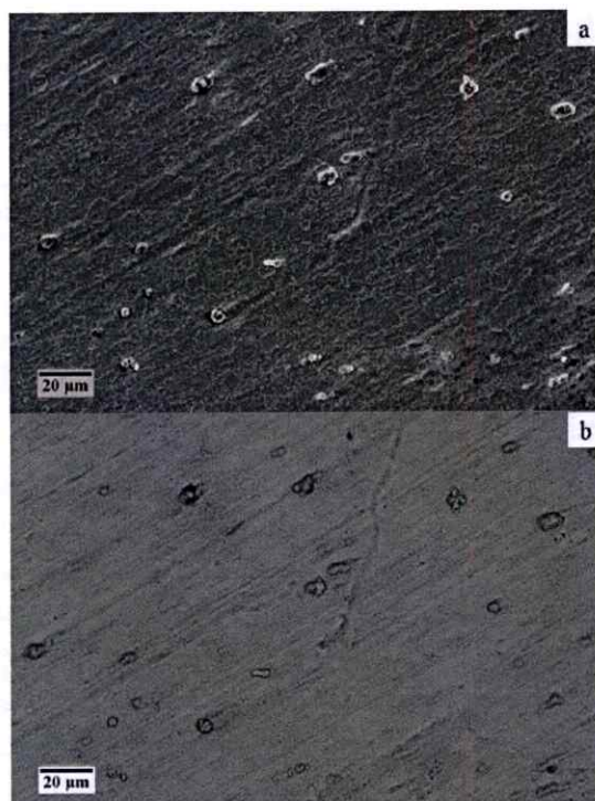
Figure 8.16 SEM images of P.CO/CO 2 -850+ox.4 at the same location in a). SE and b). BSE modes.
