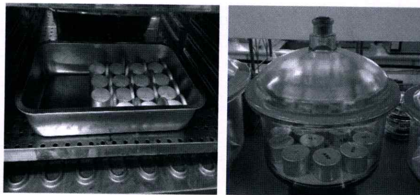
Figure 3.5 The tapioca starch moisture content measurement using standard method (Hot air oven)
