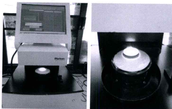
Figure 3.3 The scanning using a diode-array NIR spectrometer (DA7200, Perten, Sweden)
