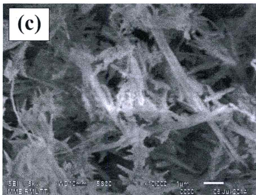
Figure 4.11 (cont.) SEM images of the as-synthesized sample prepared by hydrothermal method 130 °C for (a) 24, (b) 48 and (c) 72 h.
