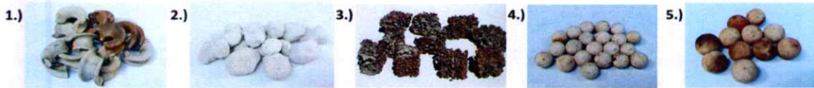
Fig. 1 Porous media material 1.) 25 mm. ceramic saddles, 2.) Random size bio-filter media from MTEC, 3.) 20x20x20 mm 3 ceramic foams, 4.) 16 mm. ceramic balls and 5.) 25 mm. ceramic balls
