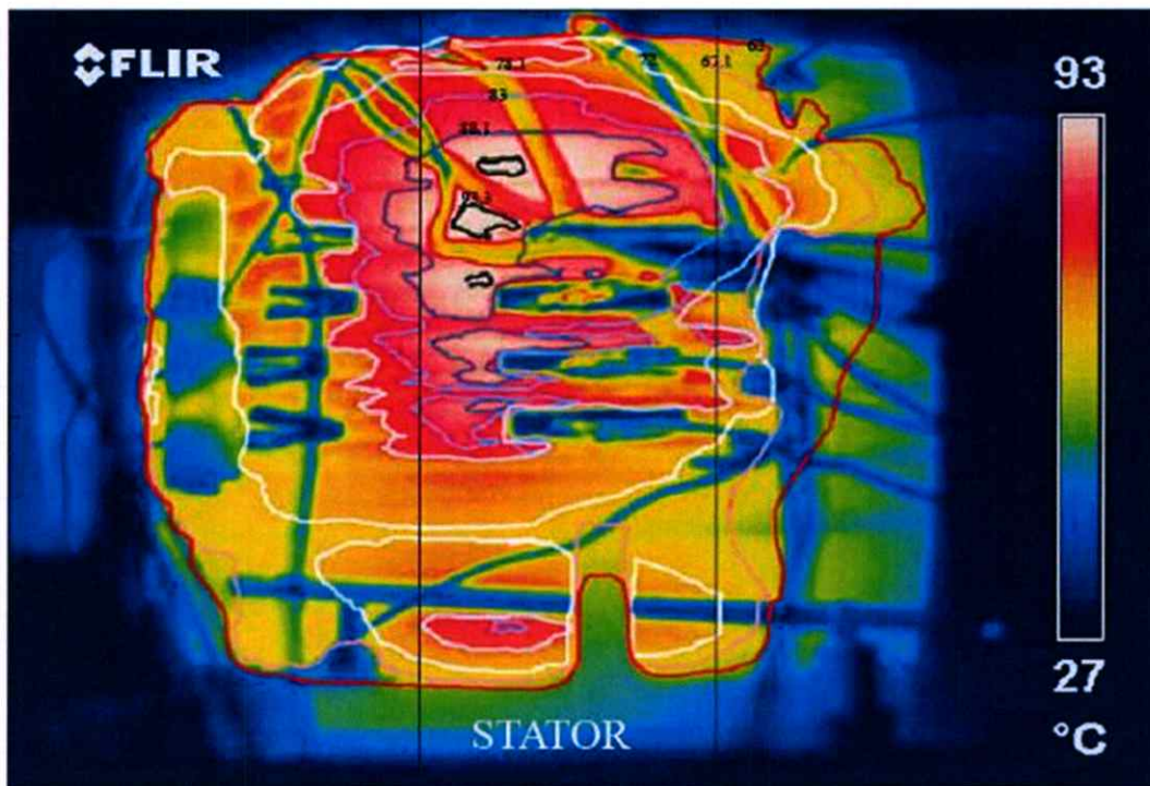
Figure 4.29 Thermogram of the 2 nd motor sample operated at 120% rated load captured at the end of the test (before unloaded)
