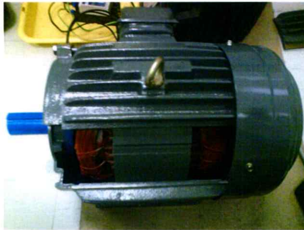
Figure 4.32 Actual test motor with cut-off housing for internal temperature measurement
