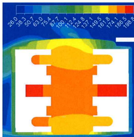
Figure 4.56 Temperature distribution around and inside TEFC motor under 120% rated load
