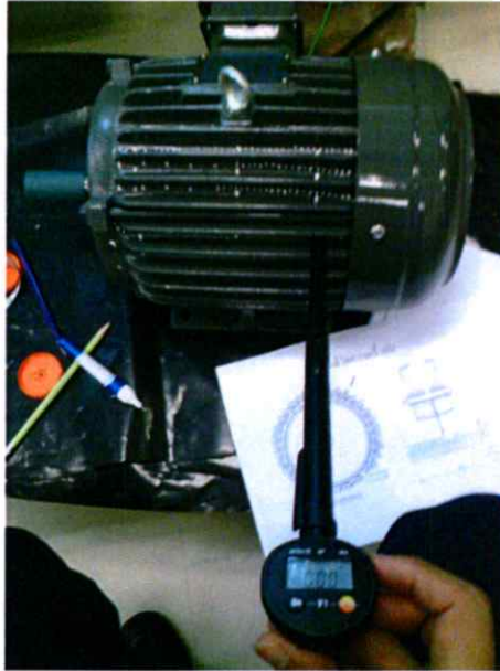
Figure 3.23 Air velocity measurement method
