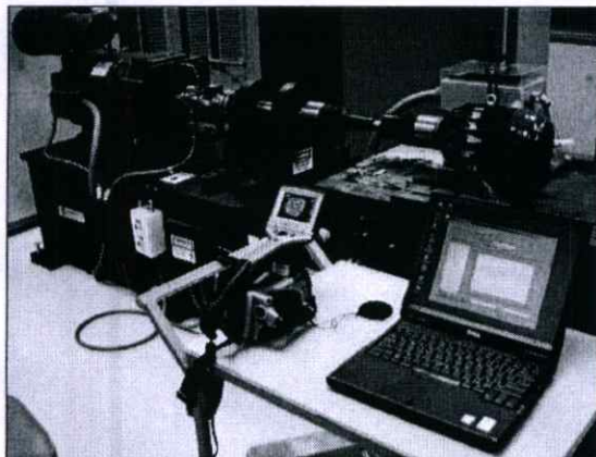
Figure 2 Experimental arrangement of the induction motor efficiency measurement
