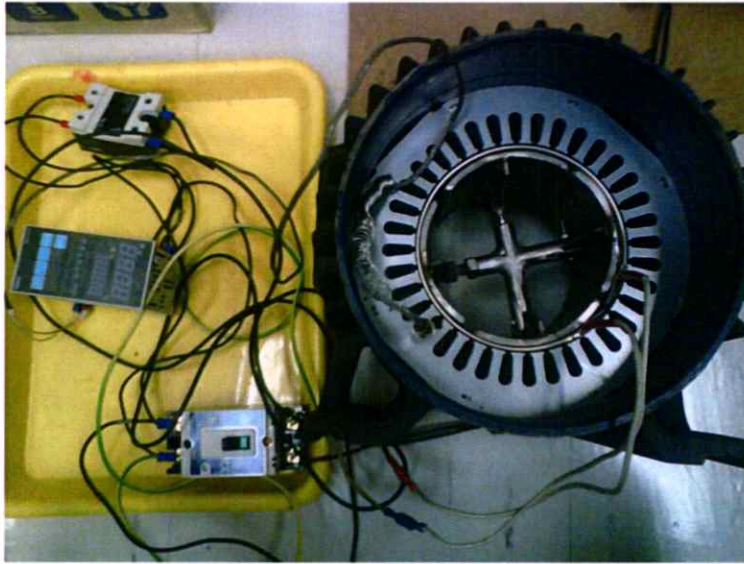
Figure 3.15 Test apparatuses configuration in an experiment to determine thermal contact resistance for stator-to-housing contact
