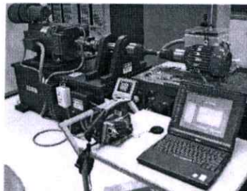
Fig.1 setup of the induction motor efficiency measurement
