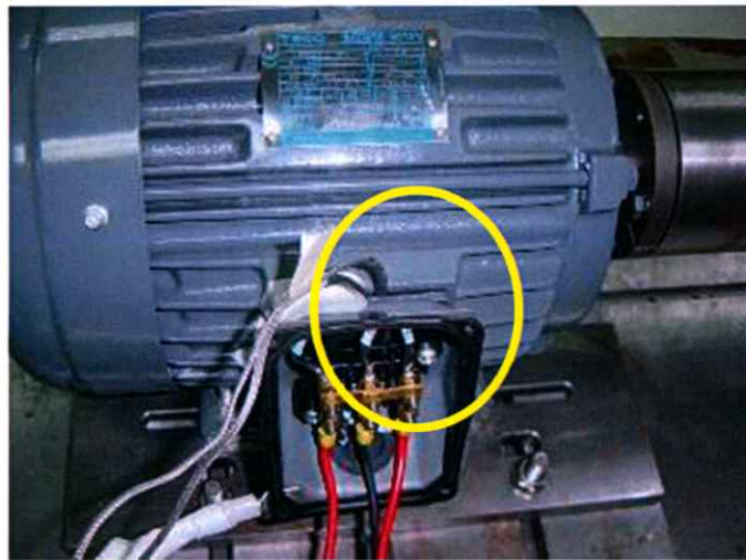
Figure 4.5 Thermocouples attachment for stator winding temperature measurement by drilling through housing
