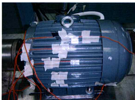
Figure 3.7 Thermocouples attachment on motor housing surface
