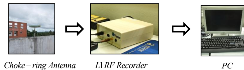
Figure 4.1: The software GPS receiver system.
