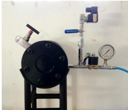
Fig. 14 Real combustion chamber including equipment
