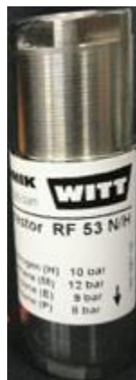
Figure 3.3: Hydrogen flashback arrestor
