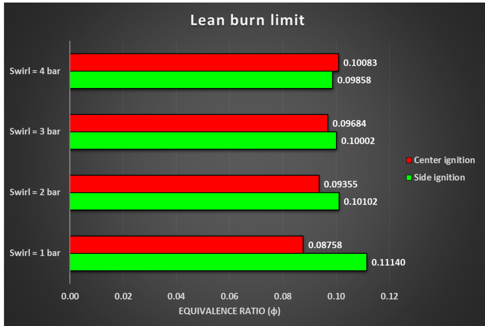
Figure 4.19: The lean burn limit result of all conditions including swirl intensity and ignition position
