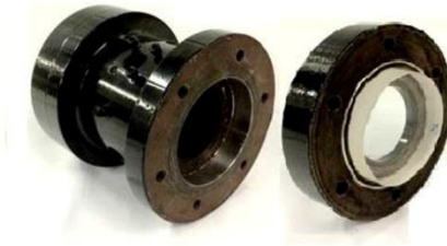
Fig. 13 Real main chamber, chamber cap and quartz glass
