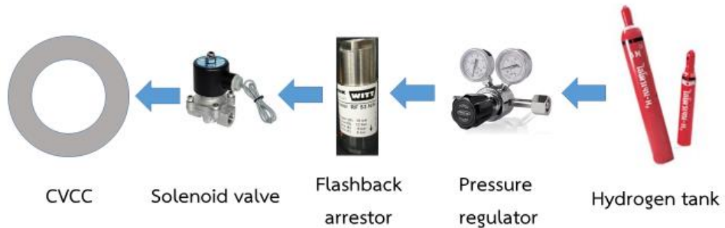
Figure 3.2: Hydrogen supply system
