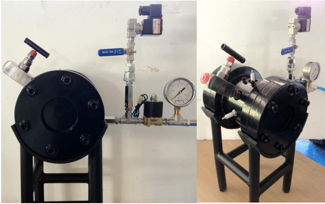
Figure 3.20: Real experimental equipment of CVCC
