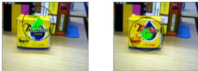
Figure 2.9 Ink box tracking use color-based particle filter (left) and hybrid Color-SIFT particle filter (right). [6]
