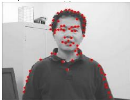
Figure 2.7 Result of Harris corner detection [5]
