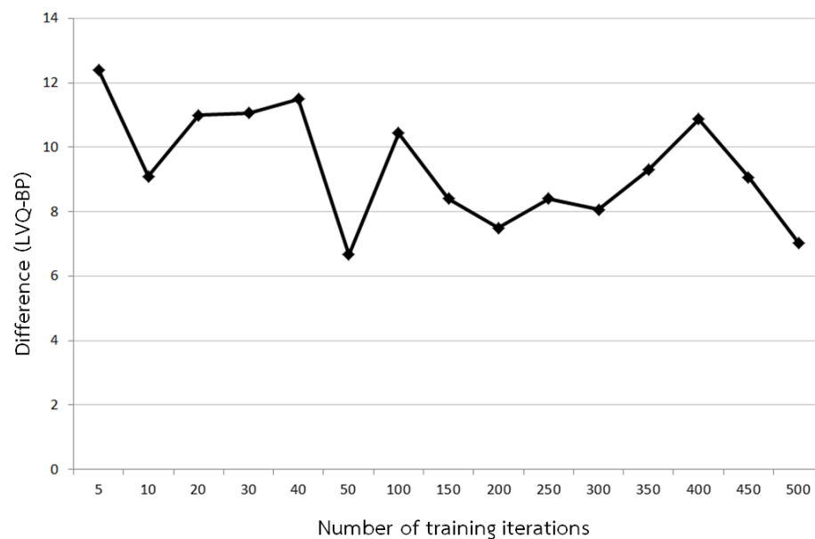
Figure 4.2: Difference of accuracy between LVQ and BP at various number of training iterations.
