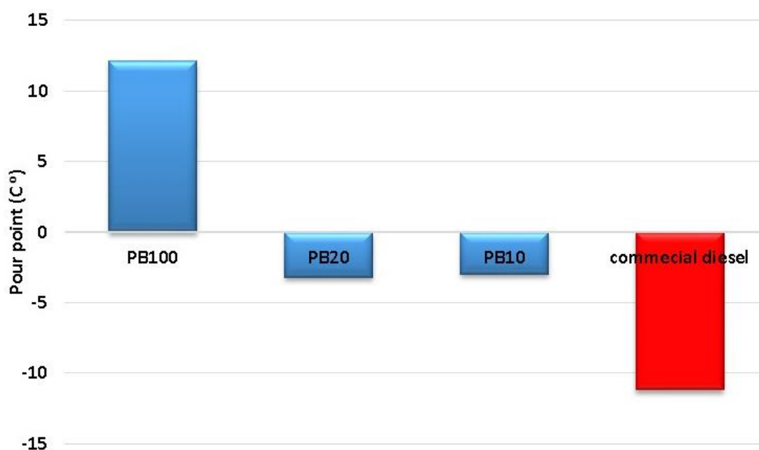
Figure 44. Results of pour point test for biodiesel fuels, blends of biodiesel fuels and commercial diesel.
