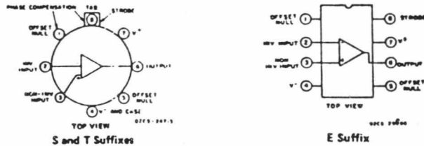
Fig. 1 - Functional diagrams for the CA3130 series.
