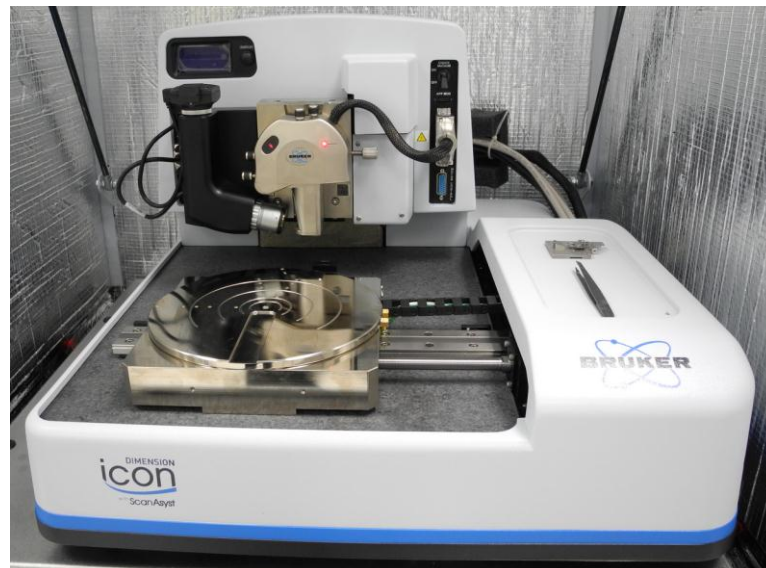
Figure 3.16 Photo of AFM (BRUKER; Dimension Icon)
