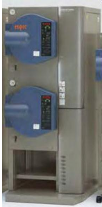
Figure 3.3 Photo of HAST Chamber (EHS - 411MD ESPEC)
