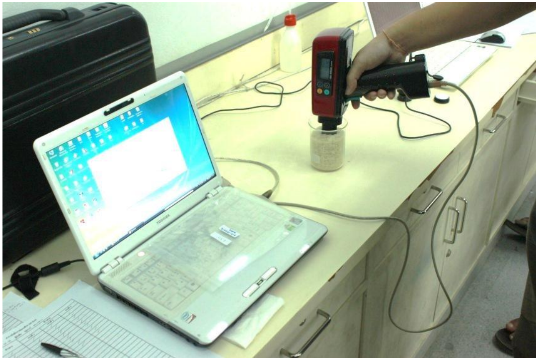
Figure 3.6 Collection of spectrum on milled rice by the short wavelength diode array (Fantec, Japan).
