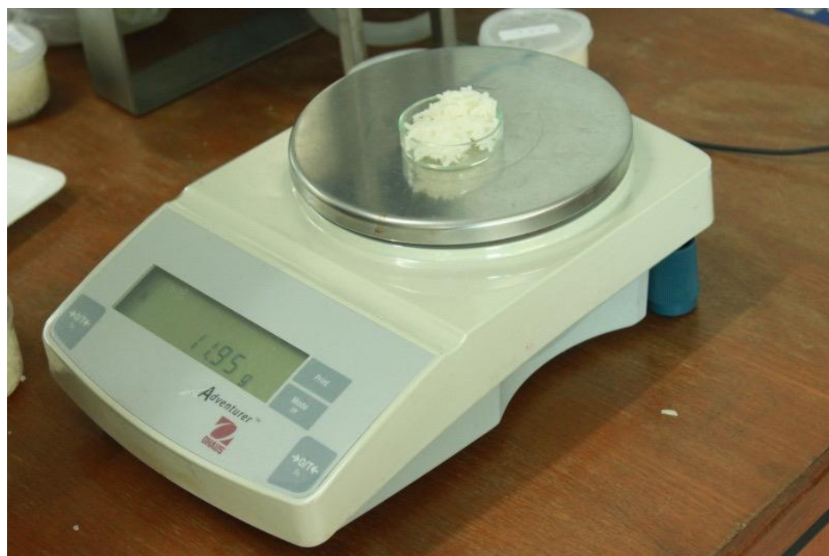
Figure 3.8 Weighting of cooked rice about 12 g on Petri dish by digital weighing machine.
