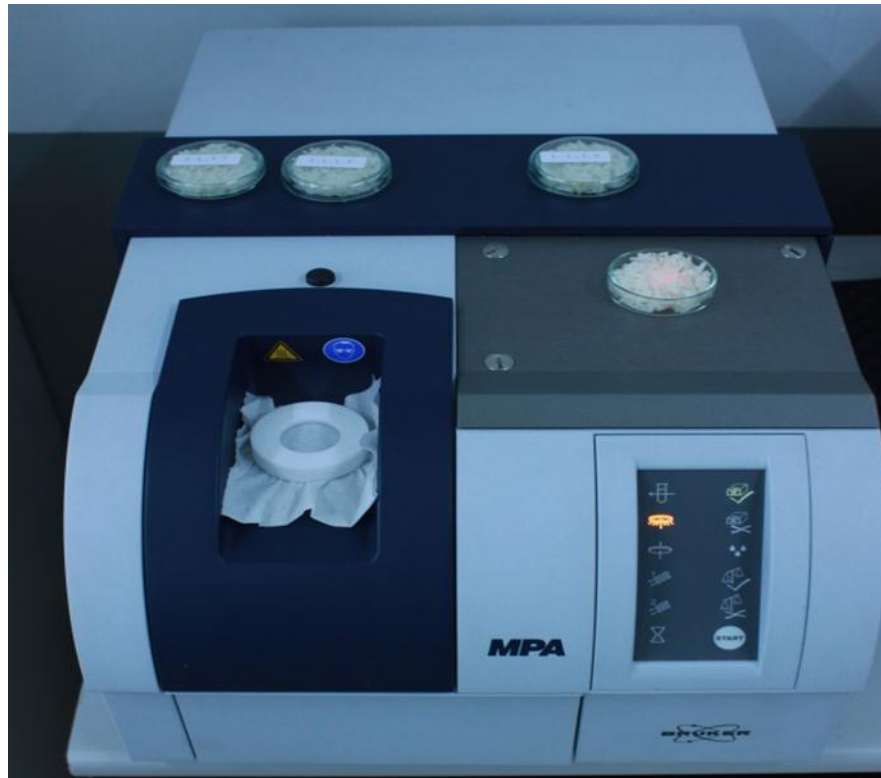
Figure 3.9 Collection of spectrum on cooked rice by FT-NIR Spectrometer (MPA, Bruker, Germany).
