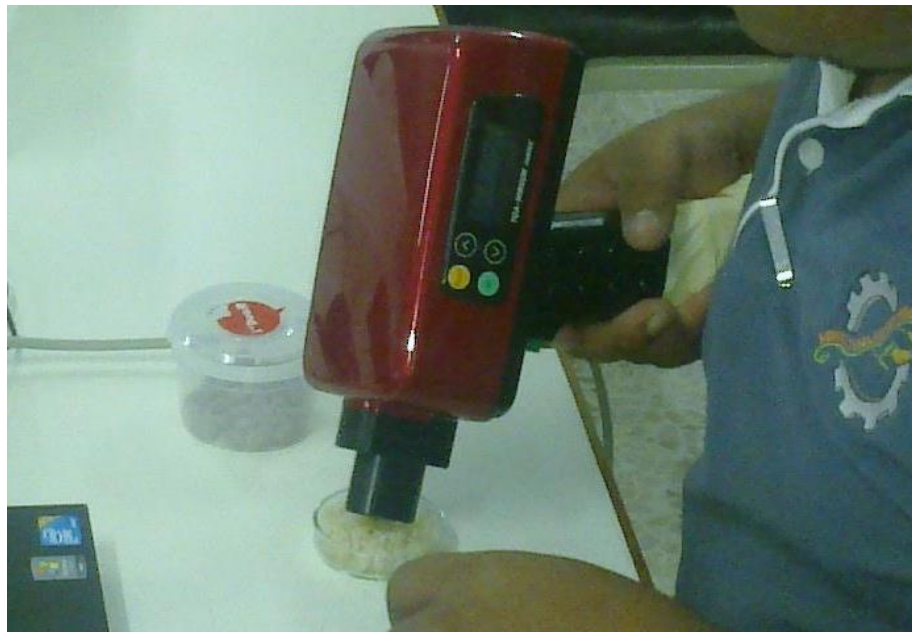
Figure 3.10 Collection of spectrum on cooked rice by short wavelength diode array (Fantec, Japan).
