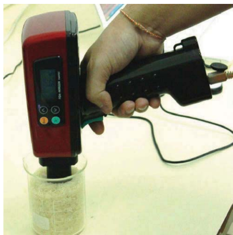
FIGURE 2 VIS-NIR spectral measurement by portable FQA-NIR GUN (FANTEC, Japan).
