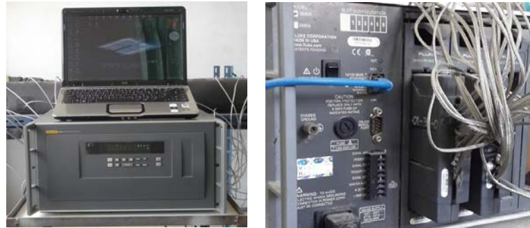
Figure 4.9 Data logger Fluke 2650A
