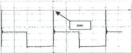
Figure 7: V_{ds} without snubber circuit 5μs/div, 100V/div
