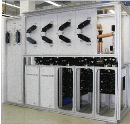
รูปที่ 2.10 CCS combiner system with combiner bypass patch panels [4]
