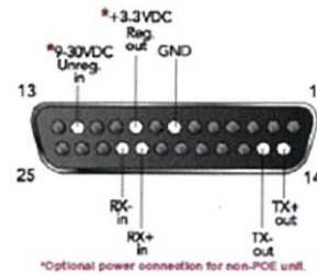
Figure B-3. DB25 Female Interface RS422 (4 wire mode)
