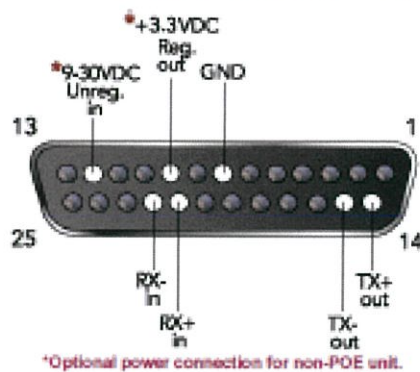
Figure B-3. DB25 Female Interface RS422 (4 wire mode)
