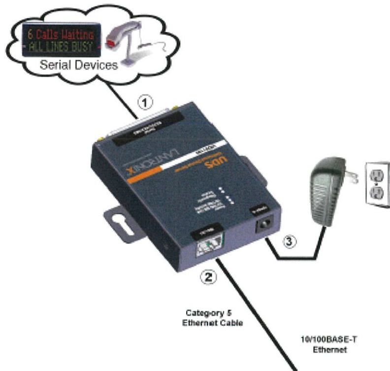
Figure 3-2. Standard UDS1100 Connected to Serial Device and Network
