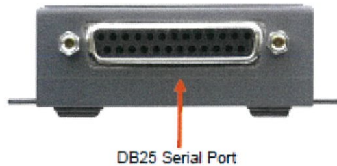
Figure B-1. Serial Interface
