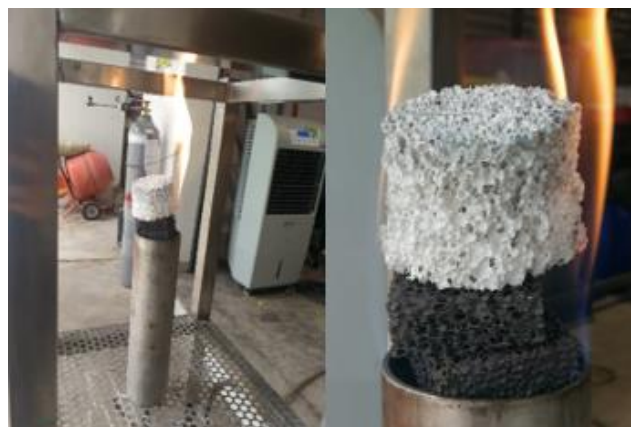
Figure 4 The combustion appears on top of burner and use that flame to preheat ceramic foam
