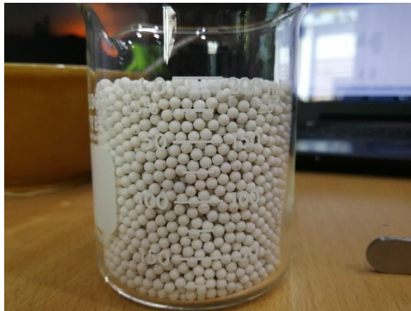
Figure 1 Put alumina balls into the beaker
