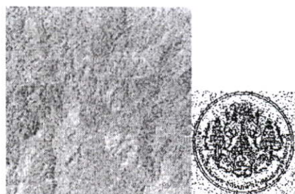
Fig. 8 Watermarked image with Gaussian noise ( mean = 0, \sigma = 0.01 ) and the extracted watermark images. (PSNR = 26.40 dB, NC = 0.7481)
