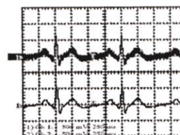
Fig. 12. Upper: ECG combined with noise frequency of 55Hz. Lower: Filtered ECG.
