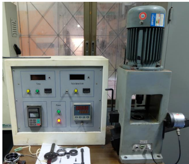
Figure 3. 4 Schematic of Four-ball wear tester followed ASTM - D4172.
