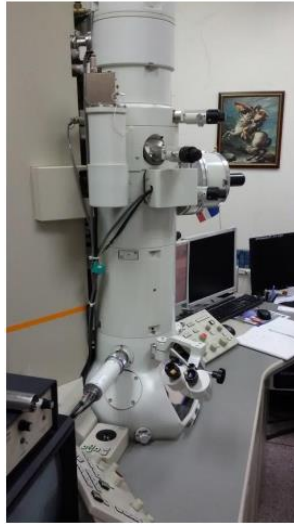
Figure 3. 2 Transmission electron microscope (JEOL JEM-2010)
