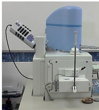
Figure 3. 6 Schematics of SEM-EDS (JSM-6610LV and X-MaxN 50).
