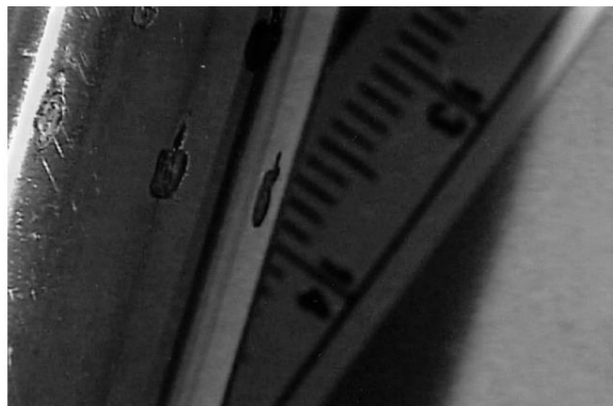
Figure 2. 14 Spalling of hard chromium on the hard steel after reciprocating [6].
