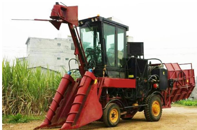
Figure 2.7 Whole stalk sugarcane harvester (FOTMA, 2019).
