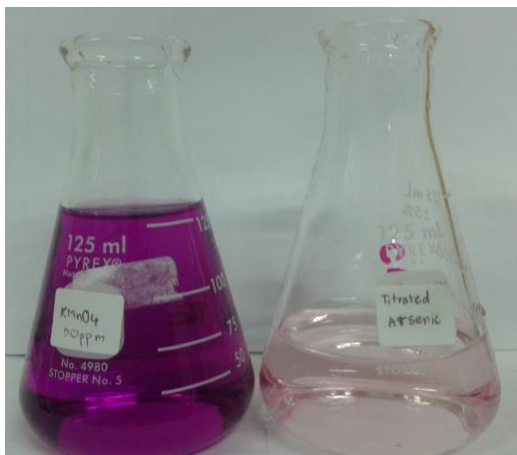
Figure 2-12 The color of \text{KMnO}_4 solution (left) and the color of end-point As(III) solution (right).
