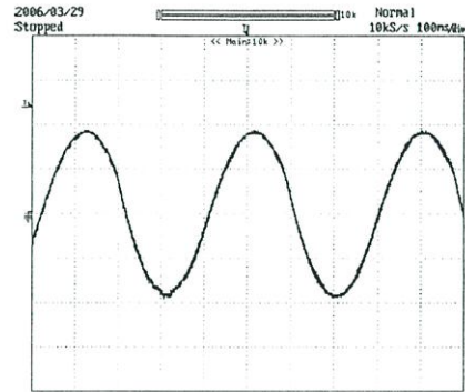
Fig.6 Response system form RNMFC to input sine.
