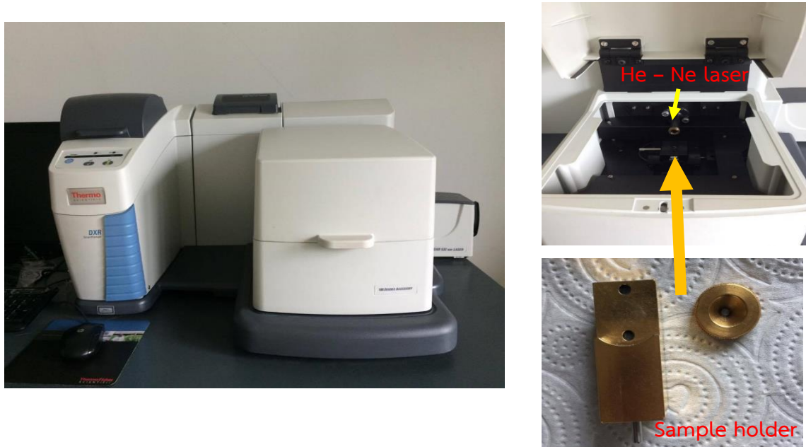
Figure 3.8 Thermo Scientific DXR Raman microscope [7]
