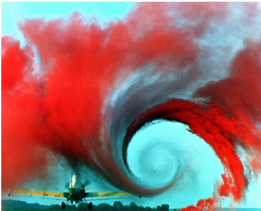
Figure 1.1: turbulence in the tip vortex from an airplane wing for chaos theory
