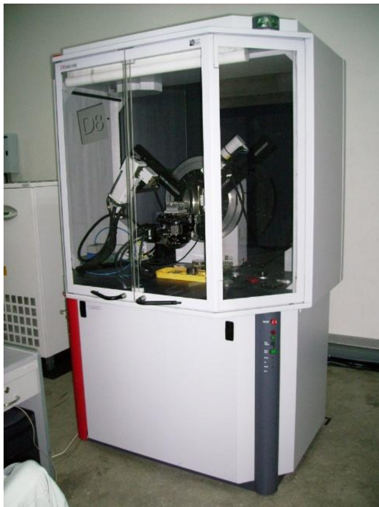
Fig. 2.11 BRUKER AXS: D8DISCOVER Powder Diffractometer [38].
