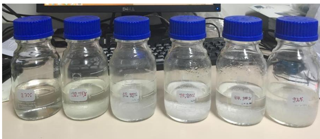
Fig. 3.6 Photograph of saturated salt solution at various level of relative humidity.
