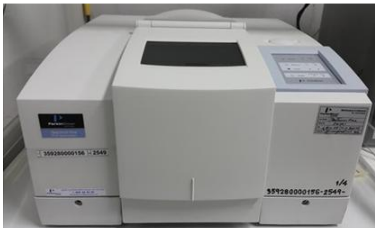
Fig. 2.14 Photograph of FT-IR Spectrometer [41].
