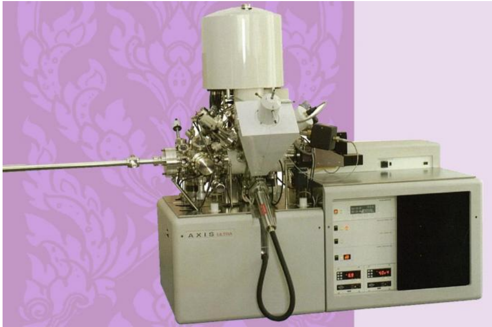
Fig. 2.16 Photograph of XPS machine [45]
