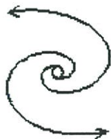
រូបទី ៣.១២ Unstable spiral node. \lambda = a \pm jb; a > 0
