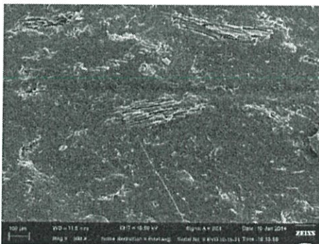
(e) +10% Sawdust particle size 50-100 mesh, 500X
