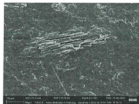
(f) +10% Sawdust particle size 50-100 mesh, 1000X
