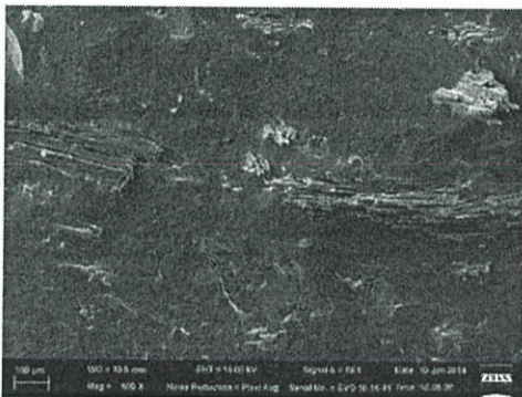
(ฉ) +10% Sawdust particle size >50 mesh, 500X
