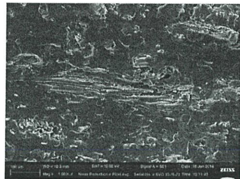
(ญ) +20% Sawdust particle size 50-100 mesh, 1000X
