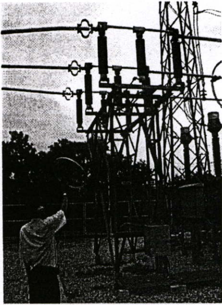
Fig. 8. Swinging the UWC to find a source of sound.
